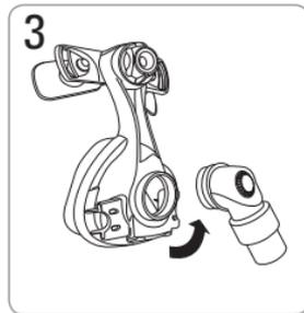
Remove the elbow assembly from the mask frame by pivoting from the bottom edge.
