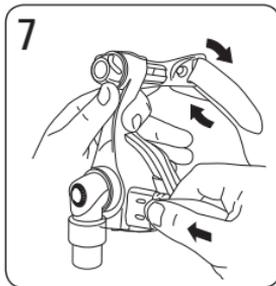
Reattach the top headgear straps by threading them through the loops.
