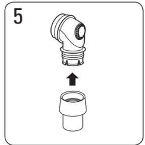
Insert the swivel into the end of the elbow.
