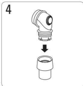
Remove the swivel from the elbow.
