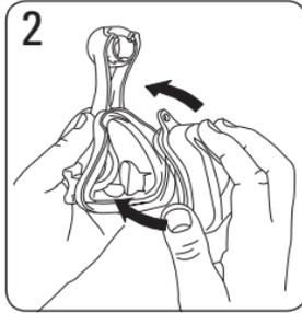
Insert the cushion into the mask frame. Ensure that the arrows at base of the cushion and mask frame are aligned.
