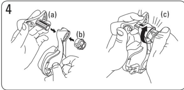
Insert the forehead support (a) into the mask frame and screw (b) the dial clockwise onto the pole. Turn the dial until it clicks (c). Ensure the dial sits flush against the frame.
