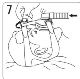
Lie down in your sleeping position. Adjust the dial until the mask is evenly positioned on your face. It should be comfortable, with a satisfactory seal. Adjust the headgear straps if necessary.
